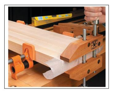
For clearance when working with small parts, clamp them in a handscrew, then clamp the handscrew in your face vise. (left)
