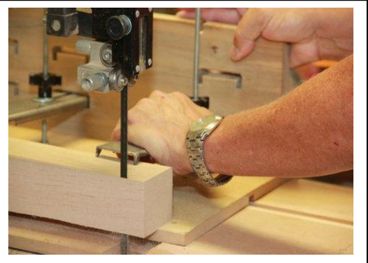
Dick Hoffmann shows how he cuts veneer strips using his shop-made band saw sled and fence.
