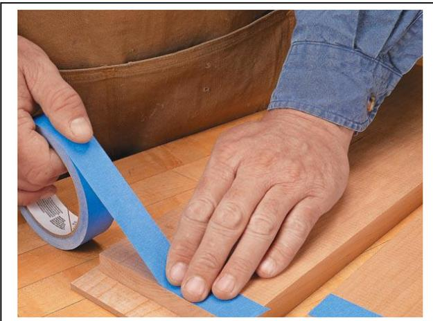
Another technique to prevent glue from sticking to the surface is to head it off at the pass. You can do this by masking off the joint before assembly. I usually only do this in a hard-to-reach area like the inside of a cabinet. I'll apply the masking tape firmly along the joint line. After the glue begins to set up, it's an easy task to peel away the glue with the tape.
