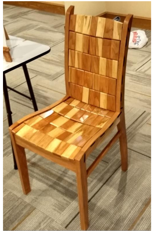
Tony Green Cherry Rope Chair (uses kevlar rope so back and seat move)
