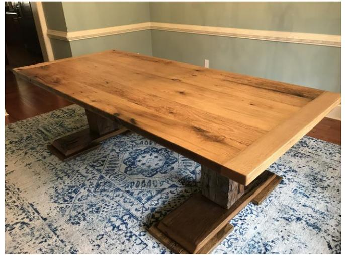
The table above was built by Daniel Taylor out of red oak support beams salvaged from 150-year-old barns in Ohio. Originally build to maintain its rough sawn character, surface instability proved impractical. Daniel devised a jig with rails to flatten the surface of the assembled table.
