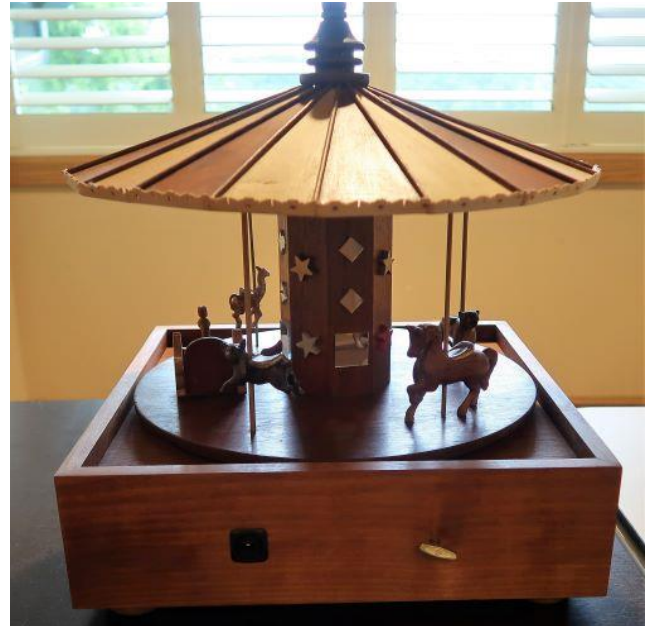
Carousel by Dennis Smith Cherry, walnut and maple construction Dremel wood carvings Used old turntable for motor
