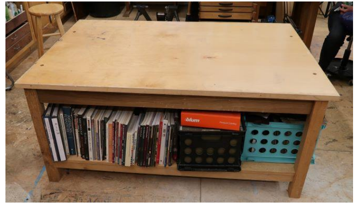
Low height work area for convenient cabinet work
