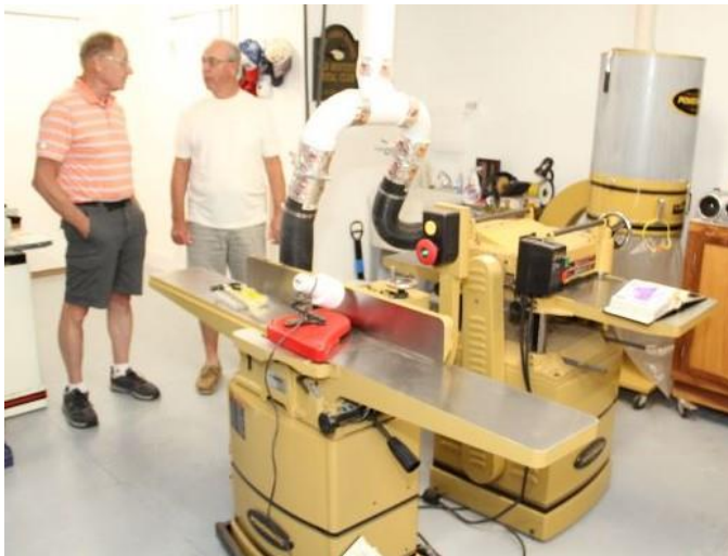
Jointer and planer setup with vacuum system
