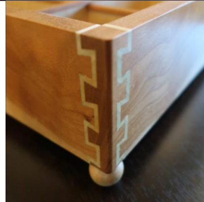
Poplar, walnut and cherry corner post dovetail boxes using an Inkra Jig by Ron Cirincione
