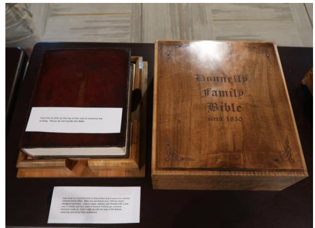
Case made by Lloyd Donnelly to protect and preserve his recently restored family bible from the 1850's. Case is maple, stained and finished with a seal coat of shellac and four coats of gel urethane. Dovetails made in the clubs Leigh jig with help of Bill McKeel; Laser lettering by Patty Authemont
