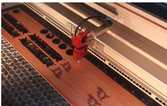
Trotec Laser Cutter and Engraver cutting miniature had saws and gears
