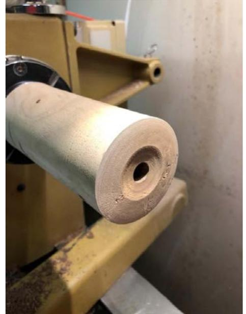
4. Using a sanding stick, sand the inside of the drilled hole until the test tube slides in easily. If you have a 9/16" drill bit, then the sanding stick will not be required. But always check to make sure the glass test tube will easily go into the drilled hole with no pressure.
