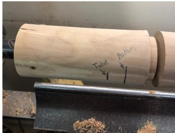
3. Remove and re-mount the wood into the 4 jaw chuck. Begin shaping the top and make a starter hole for the 1/2" drill bit. Put drill chuck in the tail stock and drill a 1/2" hole as deep as the glass test tube is long. About 5" normally. I like to leave about 1/8" of the tube sticking out of the hole when finished.
