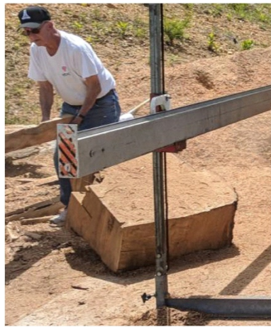
Whole end had to be cut off – Barbed wire wrapped inside
