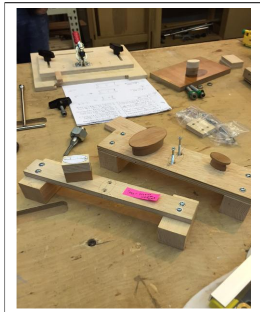
Jigs for routing small drawer pulls.
