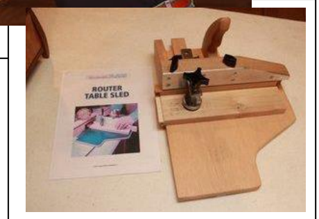
Gary Stickel describes the router table sled he made to address problems of precision and tear out in routing the ends of the rails and stiles for cherry cabinets he is building.
