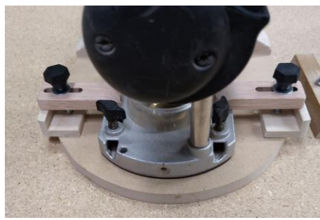
Router locking clamps that keeps the router lock to the Travel Base
