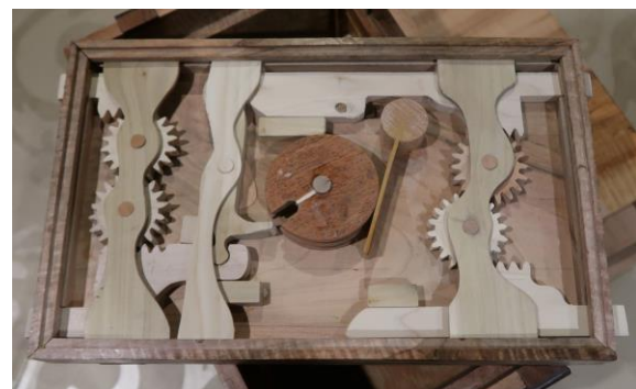
Locking mechanism in the lid of the box
