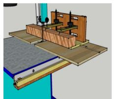
making a reference cut. The cutoff is thrown away but this reference cut establishes and edge that is now parallel to both the miter slot and bandsaw blade. Because the blade has no side pressure the cut will be true and the blade will not wonder.
