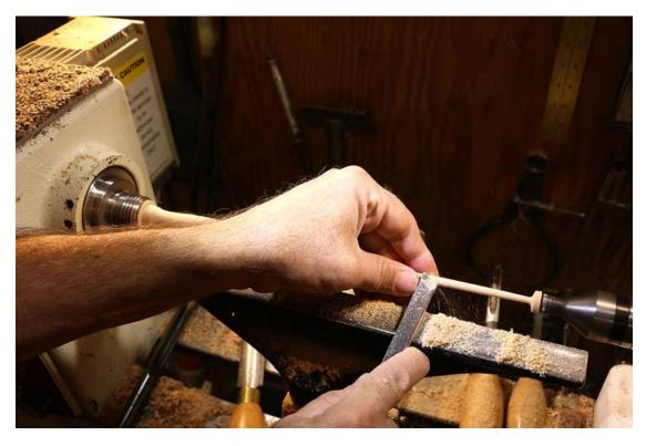
This, of course, requires holding the tool with the right hand only. I grip very near the tip and support the end of the handle by forcing it against the underside of my forearm. This supports the tool well.
