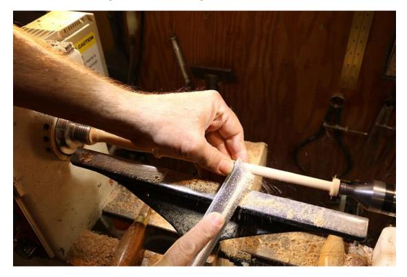
When it starts to get thin the shaft will probably start to vibrate and chatter during the cut or it may even vibrate on its own without even touching it.
