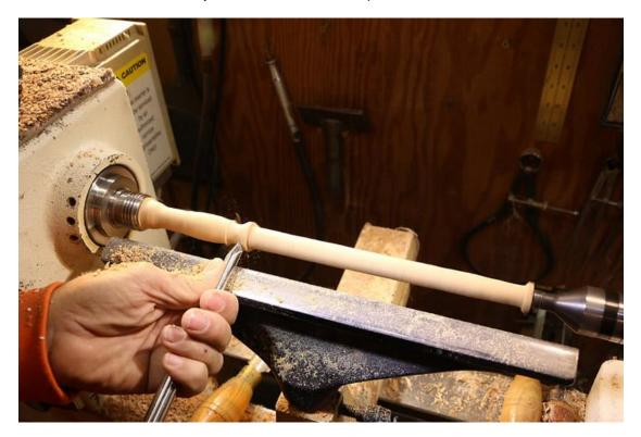
Begin tapering and shaping the shaft. I generally use a skew chisel for this. A small roughing gouge will also work. As the shaft gets thinner the fun begins.
