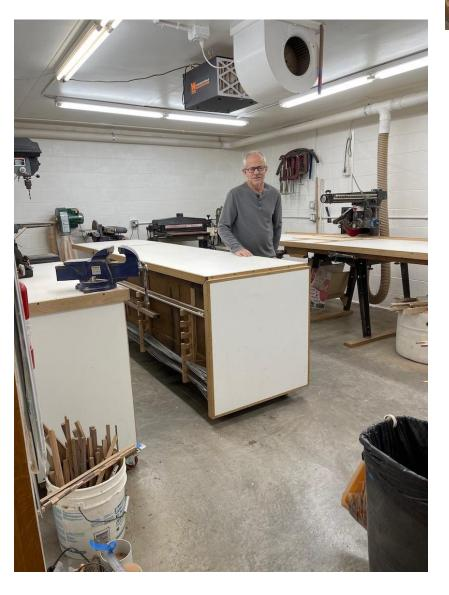
I work almost exclusively with a 12" Sears Radial arm saw, from 1970. Currently with my 3rd or 4th motor. I constructed a large 35" x 9 foot table for my RAS. The large center table has two 3' extensions and is the same height of the RAS table so I can easily manage 4x8' panel cutting.
