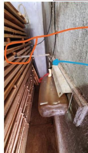
Wet Bulb Temps are measured from a temp probe inside of a wet cotton sleeve
